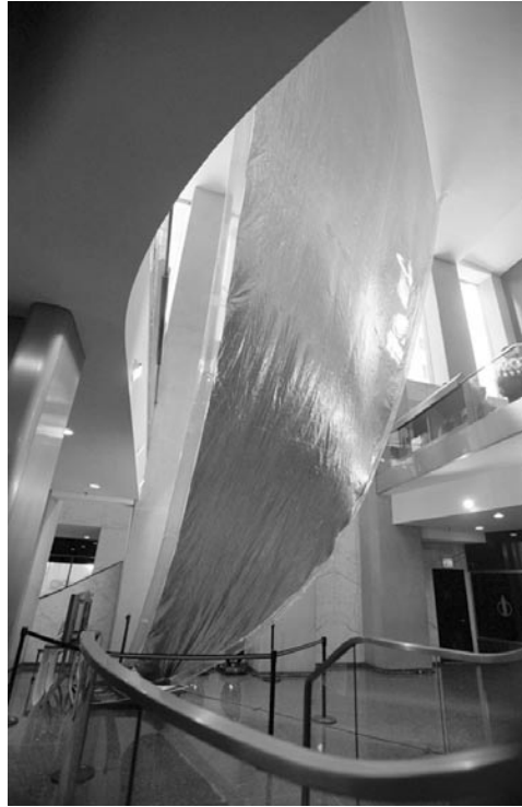
A 47-foot blade, a replica of one of eight blades that make up the Solar Sail spacecraft, is deployed in New York City's Rockefeller Center as part of a recent "Centennial of Flight" exhibit in July and August 2003. The blade gave the public its first opportunity to see this technology. Photo by Philip Greenberg, (c) The Planetary Society and Cosmos Studios.
