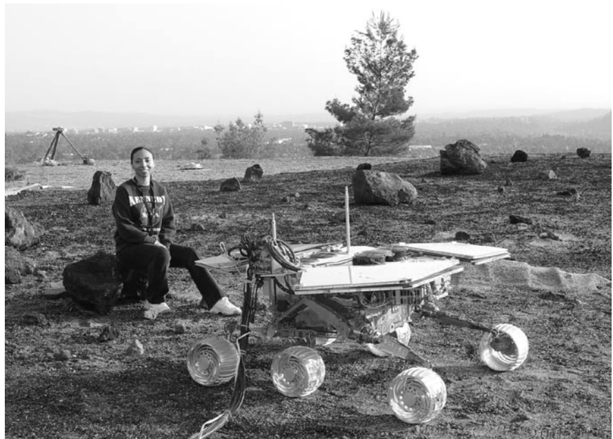
Carolina Maldonado with a replica of a rover for the Mars Exploration Rover project. The picture was taken at a location on JPL grounds, “where we set up an environment to test the rover’s mobility and navigation.”
