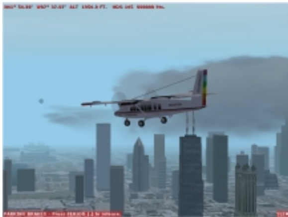
Fig. 15. An external view of the Twin Otter in Microsoft Flight Simulator, with the flight dynamics and aircraft state driven by the IEFS.
